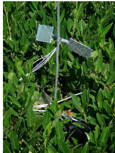
Figure 19. Heated leaf models and their installation in a canopy.
